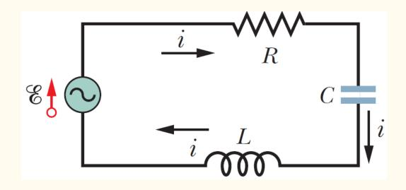
The system will oscillate at  $\omega_d$  even if its natural frequency is  $\omega$ .
