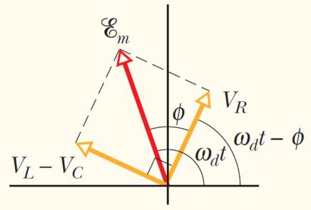
To satisfy the loop rule, the sum of the vertical projections of the phasors  $v_R$ ,  $v_L$  and  $v_C$  must **always equals** the projection of the phasor of  $\xi$
