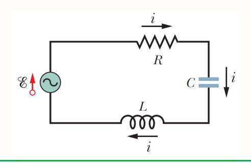
The system will oscillate at  $\omega_d$  even if its natural frequency is  $\omega$ .
