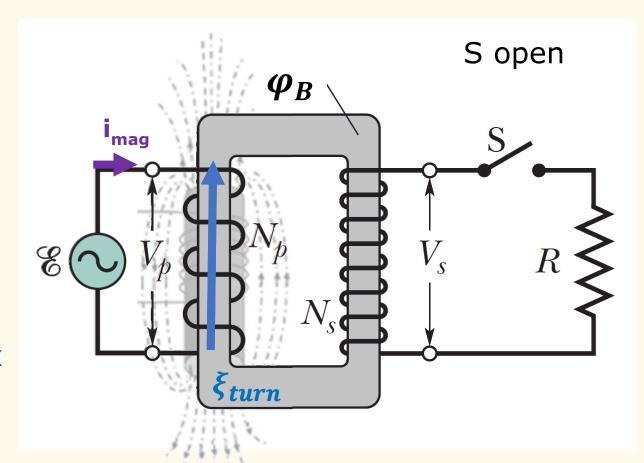
**Note:** no minus sign here to take into account the orientation of the turns with respect to the core
