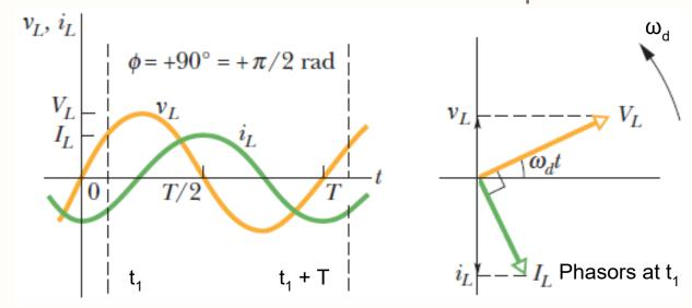
$v_L$  and  $i_L$  are one quarter of cycle out of phase  $\rightarrow \phi = +90^{\circ}$
