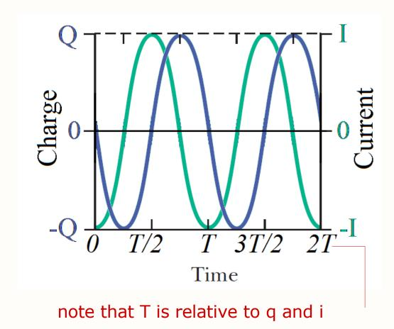
System: LC with an energy U distributed between U<sub>E</sub> & U<sub>B</sub> Assuming no losses
