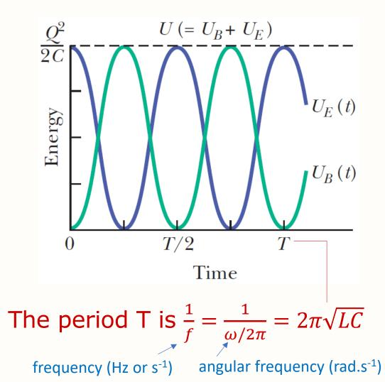
System: LC with an energy U distributed between  $U_E \& U_B$  Assuming no losses
