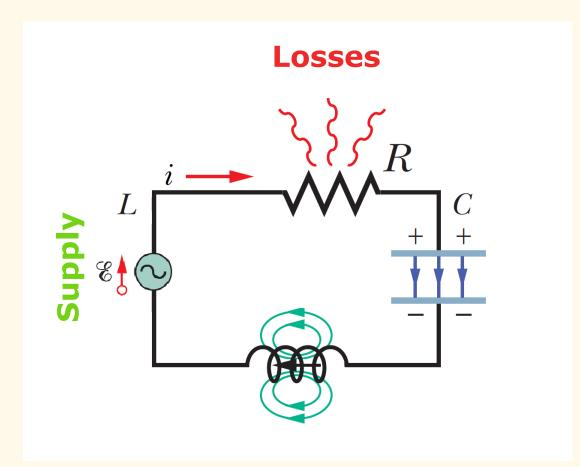
**Instantaneous** dissipated power in the resistor
