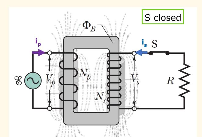
But  $V_p$  is kept at  $\xi$  by the generator  $\rightarrow$  **Produces a current I\_p to maintain V\_p**
