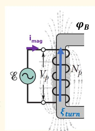
**Note:** no minus sign here to take into account the orientation of the turns with respect to the core
