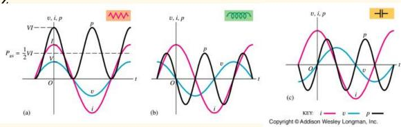
To maximize the energy transfer rate,  $\phi$  must be close to 0
